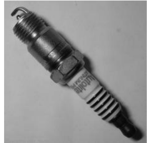
Ceramic insulator in a spark plug. The insulator is primarily \text{Al}_2\text{O}_3 , a compound of metal and non-metallic elements
